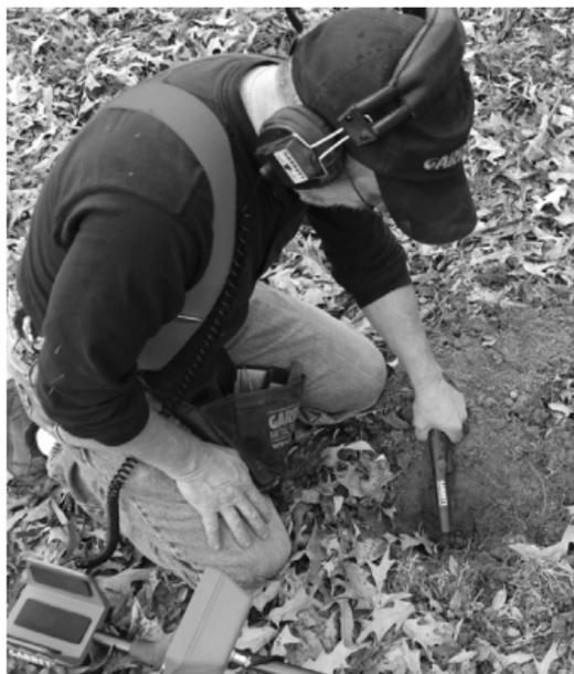
A quality hand-held pinpointer detector can save considerable time in determining if your coin is still in the ground or in the dirt pile that you have removed.
