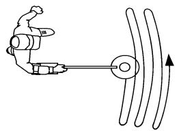
Because the loop must be moving in order to accurately respond, the sweep of the loop is critical to performance. Sweep the loop close to the ground. Keep it close throughout the sweep. Overlap each pass by at least 50%.
