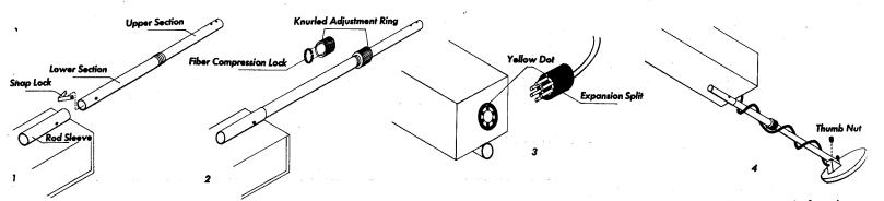
When you receive your instrument with the knurled adjustment rod, it may be necessary to install the snap lock. As illustrated in Figure Number 1. Depress snap lock and insert it in the lower section. Insert the lower section into the rod sleeve.
